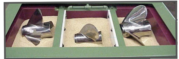
PROPS IN DRY POLISHING MEDIA. NOTE REMOVABLE TUB DIVIDERS
