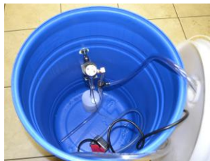
AUTOMATIC PREMIXING COMPOUND SYSTEM (cover removed)
