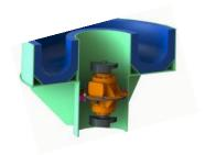
$\underline{\textit{Vibrator Motor}}$  with easily adjustable weights virtually requires no maintenance.
