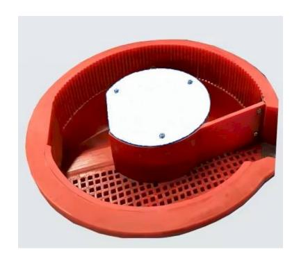
Includes parts unload system, screen and plug door. Wet or Dry operation
